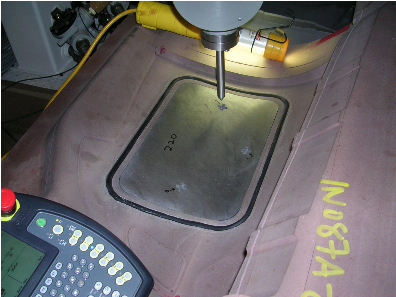
FIGURE 1: A sample part fixture. Figure shows robot with precision pointer attached, teaching Fixture Coordinate System points. The Fixture Insert was designed to have three locating features machined into it to be used at teaching points.
